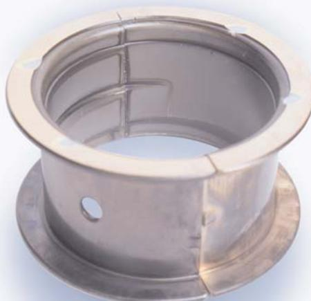
Increased crush and the elimination of flash plating improve seating of bearings in their housing for better thermal transfer from bearings to rods and block.
